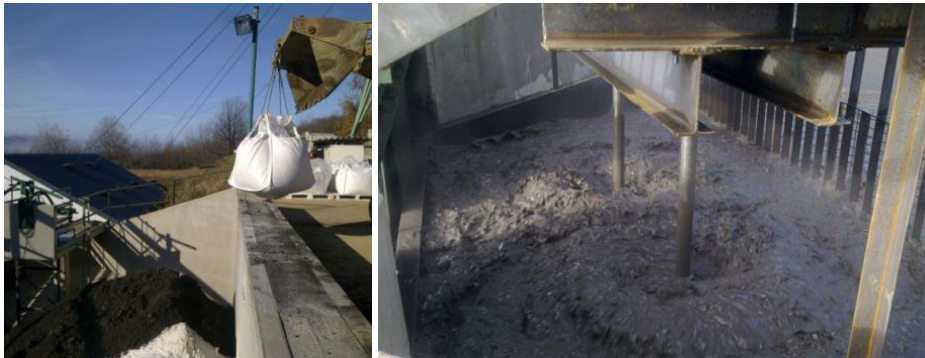
Fig. 9 Open-air lime/ash grout preparation by Mecsek Oko (Matraszentimre, Hungary)
