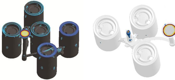
Figure 7: Is a riser needed or not? The porosity prediction for an original riserless lay-out for a grey iron grade 250 casting shows problems near the top surface (left picture). The simulation clearly demonstrates the liquid shrinkage to be the root cause of the problem. Porosity prediction for a modified layout shows that a small riser completely compensates liquid shrinkage (right picture), (pictures with friendly courtesy of ITT Water and Wastewater AB (2008))
