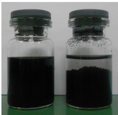
Figure 2- MWCNT/PVB/ethanol solution (left) and MWCNT-ethanol mixture with the same content of MWCNT (right)
