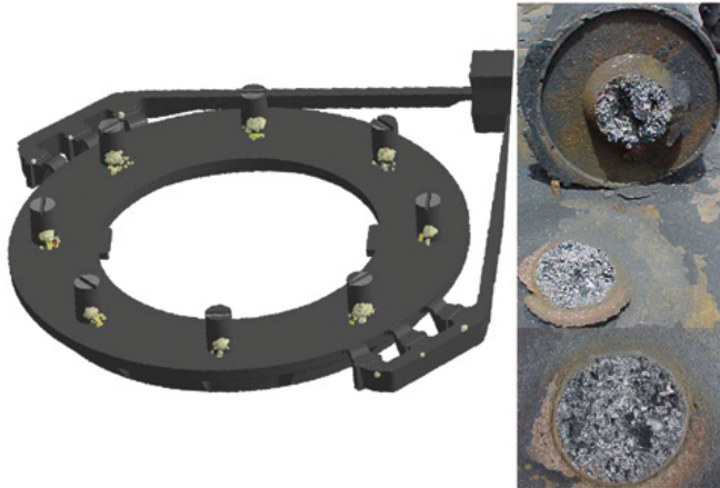
Figure 5: Predicting shrinkage in cast iron components. Secondary shrinkage below risers is shown for a ductile iron ring casting. This confirms that a simple heat flow calculation is not sufficient, as it only shows a ring shaped temperature distribution in the center of the casting. Only the combination of local shrinking and expansion behavior leads to a correct defect prediction.
