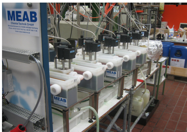
Figure 4: The mixer-settler (MSU-2.5) set-up used in the experiments.
