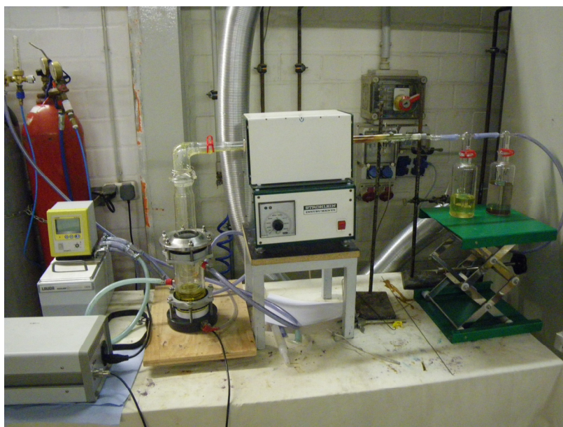
Figure 4: Experimental setup for the USP-synthesis of gold nanoparticles at IME, RWTH Aachen
