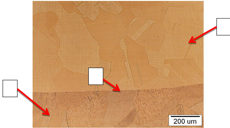
Figure 2: Optical microscopy image of internally oxidized Cu-0.4% Al sample. Arrow 1 shows the area of the oxidation zone \text{Cu-Al}_2\text{O}_3 , arrow 2 shows the area of the Cu-0.4% Al alloy and arrow 3 shows the oxidation front.
