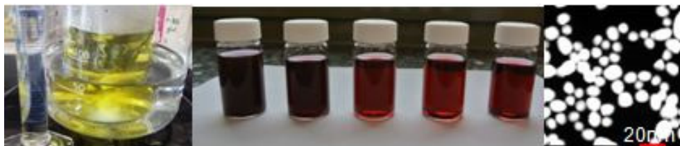
Figure 6: Synthesis of GNPs by citrate reduction and TEM analysis of GNPs
